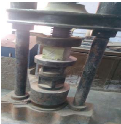
Figure 5: Compression test of prepared samples
