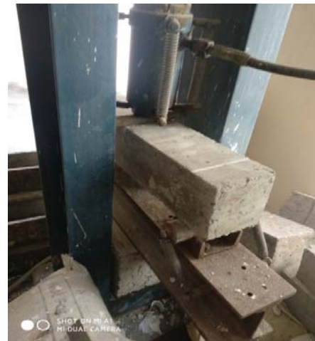
Figure 6: Flexural test of prepared samples
