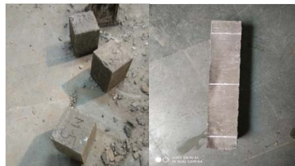
Figure 3: Fabricated samples of compression test and flexural test
