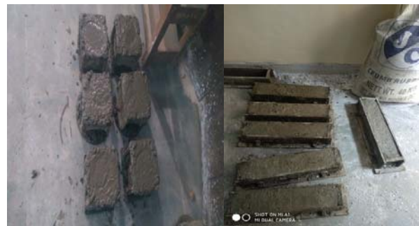
Figure 2: Mold filled with the paste of proper mix ratio
